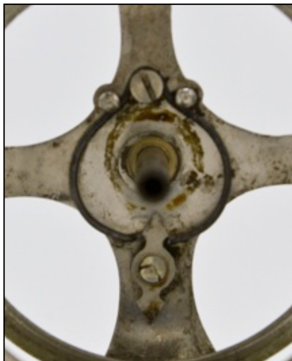
Figure 5: Close-up View of Spring and Double-ended Pawl
